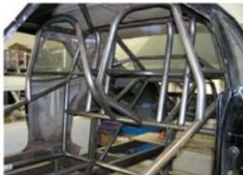
Look at the workmanship on these dual funny car cages for the interior of the Nova.
