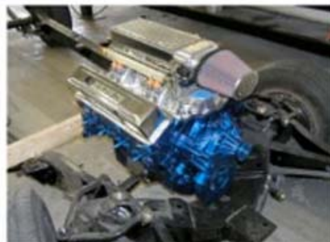
Check out this '55 Chevy chassis with 350 cubic inch engine with Holley fuel injection.
